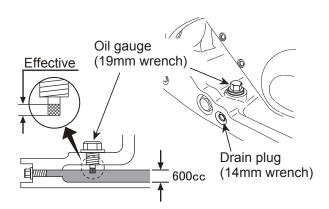
Figure 9. Vibrator Oil Check
